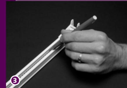
**3** Slide the second pulley onto the track (don't screw it) and mark the first ball on the opposite chain beside the pulley. This must be done on the other side of the side of operation! Take off the pulley and count eight balls (with CCS®: nine balls) from the marked one. Cut the chain after the ninth ball. Fix the master carrier overlap on the chain by following exactly the same procedure as described above.
