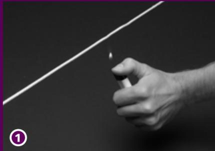
**1** Determining track-length: CKS® minus 8 cm (3,2" for center closing and one-way draw), CCS® minus 8 cm (center closing) and minus 6,5 cm (one-way draw). Determining cord-length: 2 times track length + 2 times the desired drop height of the cord. Cut the nylon cord by heating it with the lighter.
