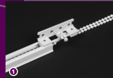
**1** Remove the metal pins inside the both pulleys. Pull the chain trough the second pulley and cross the two ends of the chain through the master carrier underlap (overlap, when it's a one-way draw). Leave two balls space after the extension of the master carrier and glue the last balls onto each other.
